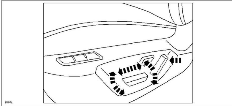
4. Slide the seat forward, then remove the rear installation bolts.
