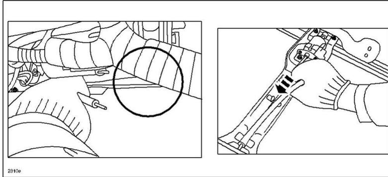
10. Pull the cable in the direction of the arrow (shown below) to remove it from the gear box.
