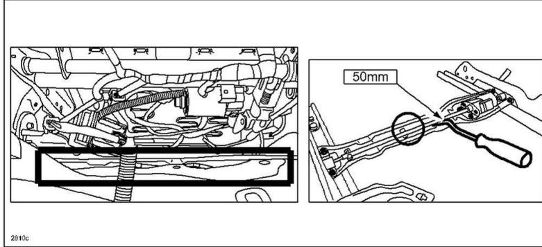
8. Hold the cable by hand and lift it up to release it from the (2) two outer cable brackets.
