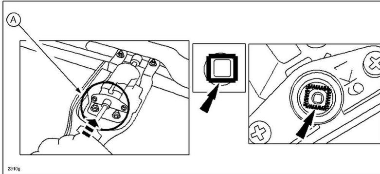
12. Align the square tip of the cable to the square shape in the gear box. Push the cable all the way in.
