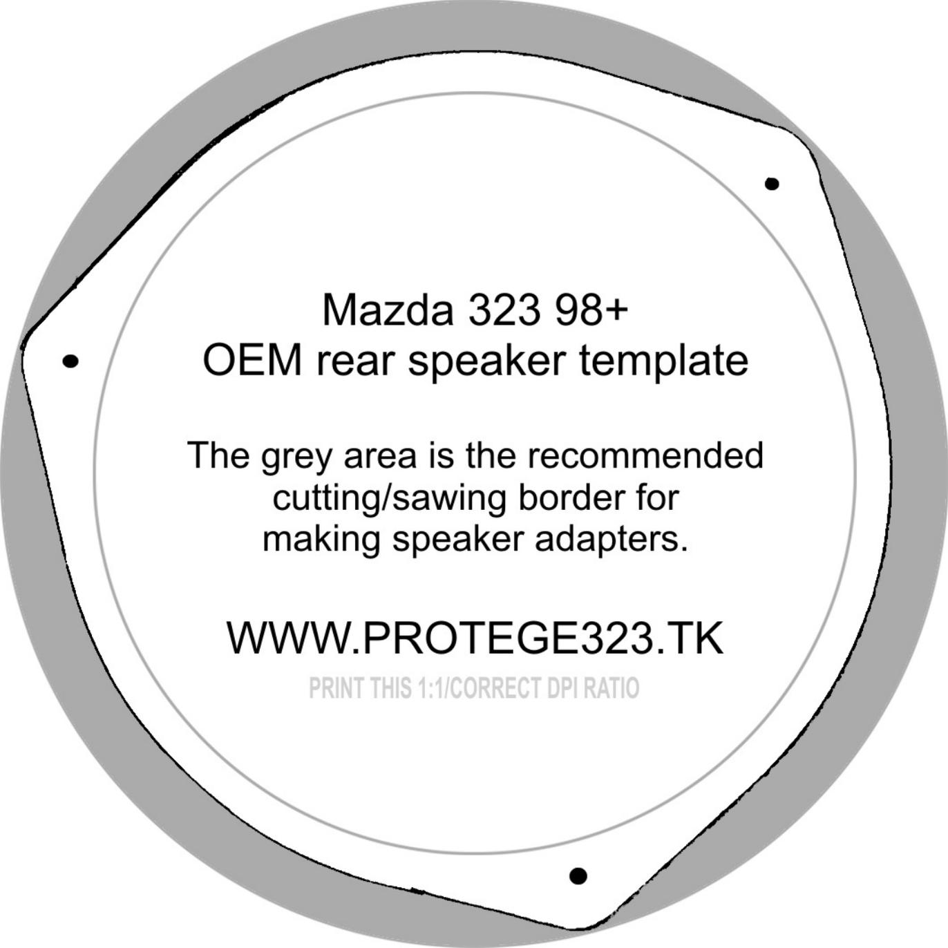
The image shows a circular template for a Mazda 323 98+ OEM rear speaker. It features a central white area with a black outline, surrounded by a grey border. Three small black dots are positioned at the top-left, top-right, and bottom-center of the white area, representing mounting holes. The text is centered within the white area.
