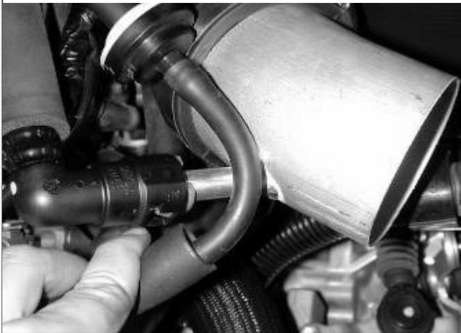
e) Attach the breather hose to the nipple on the upper pipe. The end of the breather hose will need to be rotated to fit properly.
