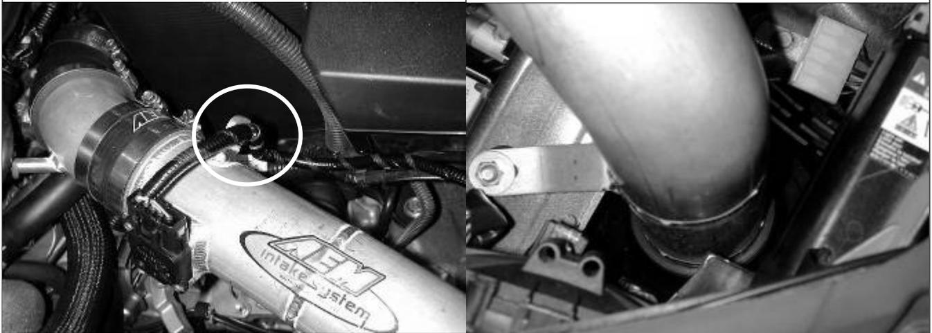
k) Plug in the MAF sensor and secure the wiring harness using the supplied tree mount zip tie. Trim the excess plastic zip strap. Reinstall the plastic intercooler cover removed in step 2a.
