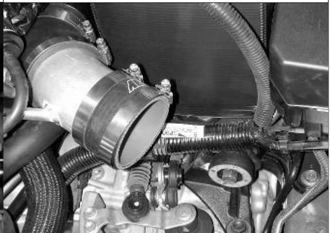
f) Install the 3" coupler to the end of the upper inlet pipe. Secure the coupler with a #48 hose clamp.
