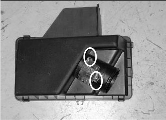
k) Remove the two screws securing the MAF sensor to the air box lid. Be careful not to damage the sensor.
