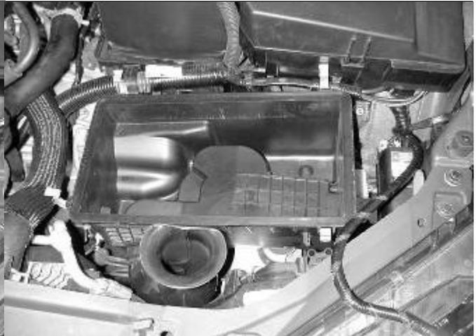
f) Remove the stock air filter. Next, pull up on the lower air box housing and remove it from the engine bay.
