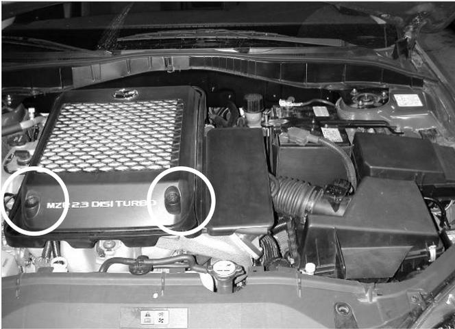
a) Before removing any of the O.E. components, **label each individual part so that no components become mixed up during the installation process.** Remove plastic intercooler cover by removing the 2 bolts securing it to the intake manifold.
