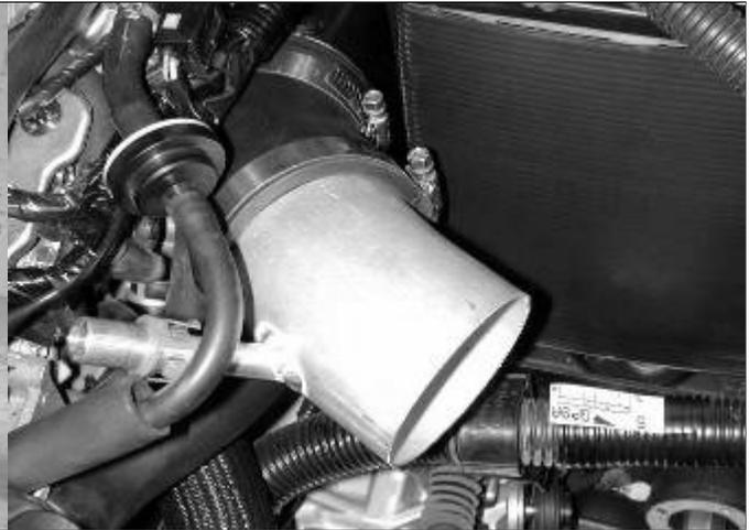
d) Slide upper inlet pipe into the previously installed coupler with the breather nipple angled towards the engine. Secure with a #48 hose clamp.
