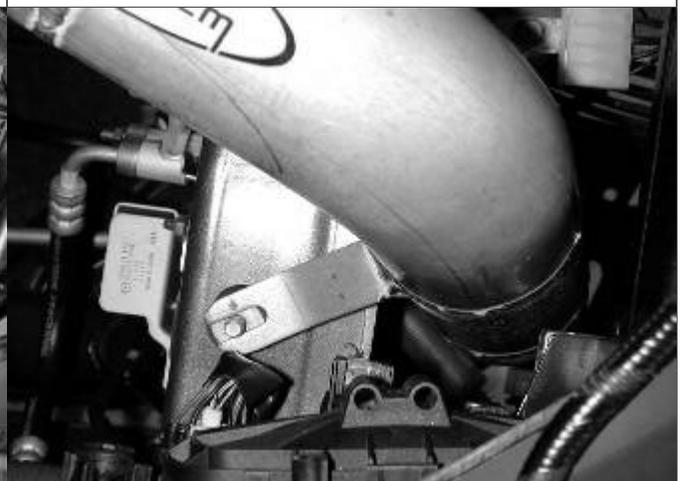
h) Install the lower inlet pipe into the coupler attached to the upper inlet pipe and use a #48 hose clamp so secure. Align the intake mounting bracket with the rubber mount installed in previous step.
