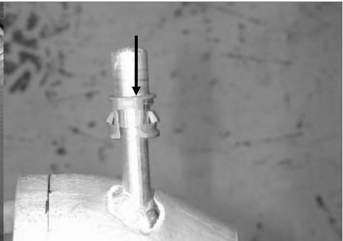
b) Check to see that the inside of the **AEM CAS** pipes are clean and free from any foreign objects. Install the previously removed blue plastic breather hose retaining clip by carefully sliding it over the breather hose until it snaps into place.
