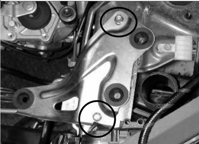
g) Remove the two bolts securing the lower air box mount to the vehicle chassis and remove the mount.
