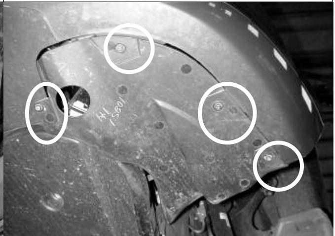
h) From underneath the vehicle, remove the 4 screws and two plastic connectors securing the inner fender liner to the bumper.
