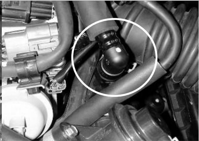
b) Disconnect the plastic breather hose from the inlet tube. This is done by squeezing the blue retaining clip and pulling on the breather hose.
