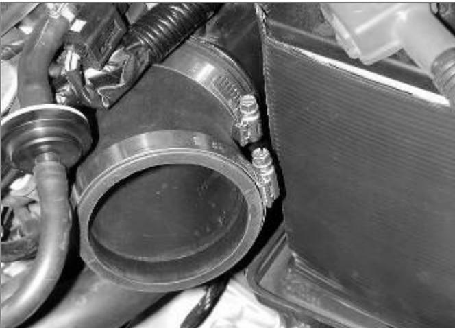
a) Install the 45 degree coupler onto the turbo inlet tube and secure using a #40 hose clamp.
