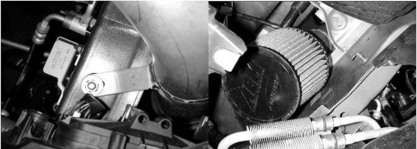
i) Secure the lower inlet pipe using the supplied M8 washer and nut.
