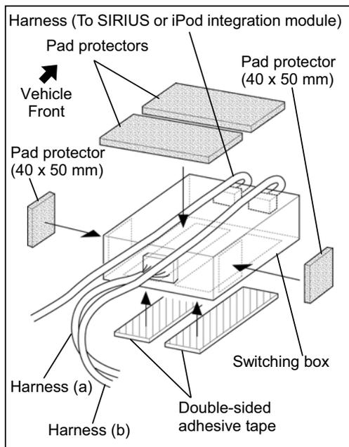
1. Peel the backing of the double-sided adhesive tape and affix the tape to the switching box.
