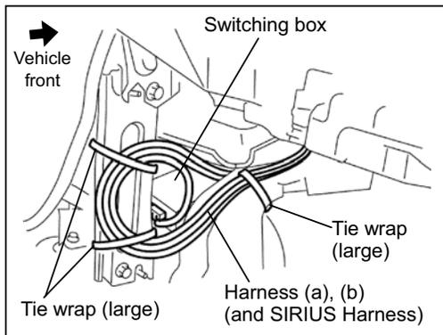
12. Secure excess wiring harness, wiring harness (a) and (b) (and SIRIUS harness) with tie wraps (large).
