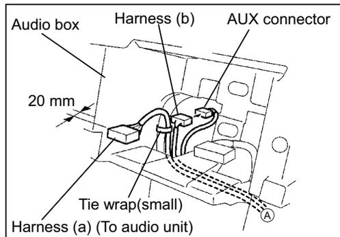
8. Pull the harness (a) 16-pin connector 20 mm out from the audio box.
