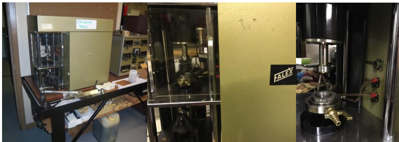
Figure 2. Bench test apparatus configured for the Four-Ball Wear Test. Industry standard for evaluating and optimizing the wear prevention characteristics of different lubricant formulations. The testing platform is a Falex Multi-Specimen Friction and Wear Test Machine.
